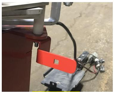
A) Next, place part number 120100584 on the inside of the small mounting bracket as shown below and use the following hardware numbers HDW2050 & HDW2020 to fasten the mounting bracket to the mating part.
