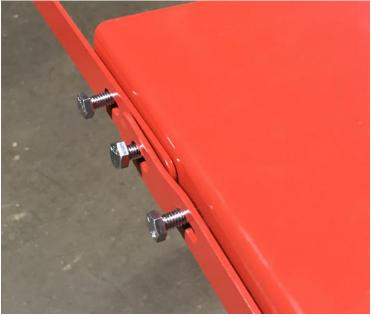
*10) Lastly attach the front guard support using three HDW2020's to the HDW2087 as shown below.*
