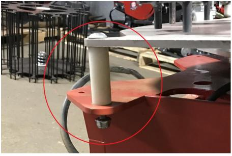
2) Place the larger of the two brackets (part number 120100582) on the bottom side where the nut was just removed. Fasten the bracket to the frame using hdw2020 that was removed in step 1. NOTE: The larger mounting bracket must be placed on the SAME SIDE of the frame that the throwing plate extends out on.
