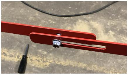
8) Next remove the two nuts under the throwing plate that mount to the frame as shown below. Then place part number 120100597 underneath the frame and tighten to frame using the two nuts we just removed.
